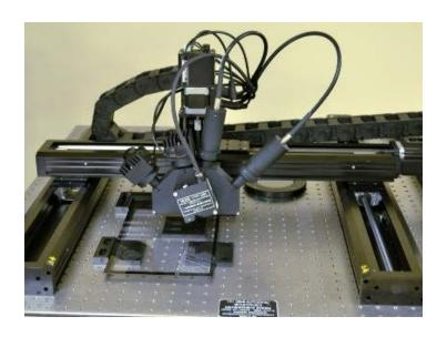
The GS-191SA-1045 is a manually loaded gonio-reflectance measurement system that automatically captures complete spectral & colorimetric properties for coated glass, polished substrates or diffuse surfaces at 0° and 45° angle of incidence simultaneously, without requiring second-surface masking. Substrates as thin as 500  $\mu m$  can be tested with typical scan times of 200 msec per measurement point.
