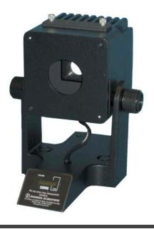
The RS-10D is a precision source of radiant flux, used primarily to calibrate light-measuring instrumentation and as stimuli to measure detection devices. To maintain constant output, tungsten halogen lamps are used exclusively in combination with ultra-stable constant-current supplies incorporating shunt current measurement and comparison circuits.
