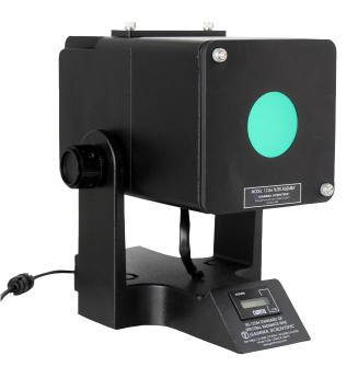
The RS-12DN is a NIST Traceable source that can be used as a white light standard of spectral radiance or luminance. The insertion of the filter/aperture assembly transforms the unit into an NVIS display simulation source approximating a green cockpit display with a designed level of near infrared output against which a spectroradiometer or radiometer can be calibrated.
