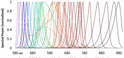
SpectralLED® Tunable Light Source LED Spectral Power Distribution
