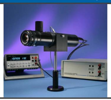
The TIA-3000 series consists of a high performance transimpedance amplifier with dark current levels as low as 3 femto-amps, superior blue light sensitivity and highly accurate measurement capability in terms of wavelength, color and power. Standard configurations include Si, InGaAs with temperature stabilized configurations available.
