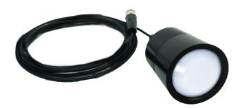
The Model 211 Photometric sensors are designed with spectral responsivity that matches the human visual response, incorporating a silicon detector combined with a spectrally matched photometric filter. An integrated cosine filter significantly reduces directional sensitivity for ease of use.
