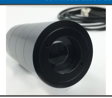
The model 2153V-12.5 is our standard Luminance sensor with an integral lens that provides a fixed field of view (FOV) of 12.5 degrees\*. It is ideally suited for measurement of the brightness of diffuse surfaces or uniform light sources, such as the intensity of displays.
