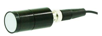
The model 263 miniature Photometric sensors are designed with spectral responsivity that matches the human visual system, incorporating a silicon detector combined with a spectrally matched photometric filter. An integrated cosine filter significantly reduces directional sensitivity for ease of use.
