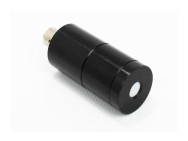
The model 264 radiometric sensor is our miniature series silicon sensor specifically designed for laser power measurement. It contains an integrated diffuser and reduced aperture for attenuation of optical power.
