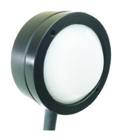
The model 268P is a low-profile illuminance sensor designed for applications with limited mechanical clearance. These Photometric sensors are designed with spectral responsivity that matches the human visual system, incorporating a silicon detector combined with a spectrally matched photometric filter. An integrated cosine filter significantly reduces directional sensitivity for ease of use.
