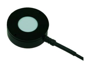
The model 268UVA is a low-profile sensor designed for applications with limited mechanical clearance. The unit is optimized for 365nm measurement in the UVA portion of the spectrum (320-400 nm) via an integrated filter, and provides Irradiance measurements in W/cm<sup>2</sup>.
