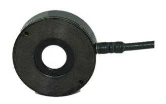
The model 268 UVC is a low-profile sensor designed for applications with limited mechanical clearance. The unit is optimized for measurement at 254nm in the UVC portion of the spectrum (200-290 nm) via an integrated filter, and includes a diffuser to provide Irradiance measurements in W/cm<sup>2</sup>.
