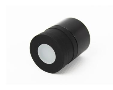
The model 3211 Photometric sensors are designed with spectral responsivity that matches the human visual response, incorporating a silicon detector combined with a spectrally matched photometric filter. This matched photometric filter and cosine diffuser lowers the error in spectral matching, particularly in the blue and violet portion of the spectrum. The integrated cosine filter significantly reduces directional sensitivity for ease of use.
