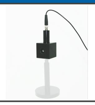
The model S2575 Integrating Sphere consists of a model 260 silicon sensor coupled to a model 2575, 50 mm diameter integrating sphere. The unit provides measurements in W or mW.
