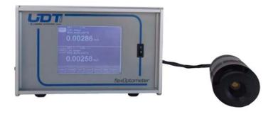
The C Series Optical Meters include an integrated controller that is compatible with our thermo-electrically cooled silicon and indium gallium arsenide (InGaAs) detectors. This feature results in an order of magnitude greater sensitivity than standard Optical Meters, resulting in outstanding performance when measuring low light levels.
