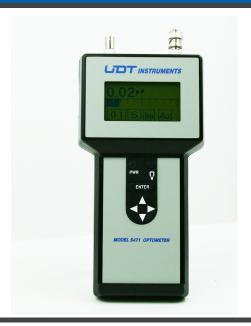
The model S471 High Performance Handheld Optical Meter is ideal for photometric, radiometric, laser power, and fiber optic measurements. Designed to be used in a laboratory setting or field environment, the microprocessor controlled architecture features direct analog display, serial RS-232 output and analog voltage output.
