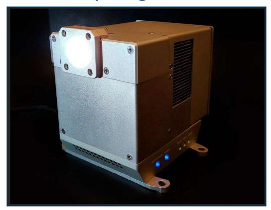
ISTEQ's XWS-30 light source product has been specially developed for those customers, who needs super compact broadband light source with low heat dissipation, keeping the plasma brightness high.
