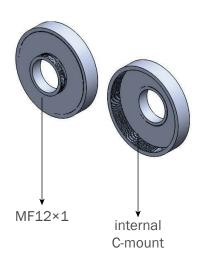
$MF12 \times 1 \rightarrow C$ -mount (internal thread)
