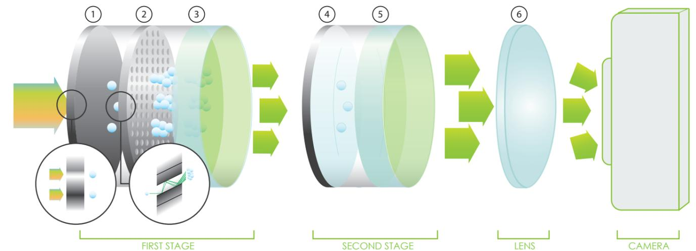
On the photocathode(1) photons get converted into electrons. These are accelerated in an electric field towards the Multi Channel Plate (MCP, 2) and hit the channel walls. Depending on the voltage across the channel, multiple electrons are generated by secondary emission. This cloud of electrons gets accelerated towards the anode screen (3), where the electrons are converted back into photons by the phosphor layer.
