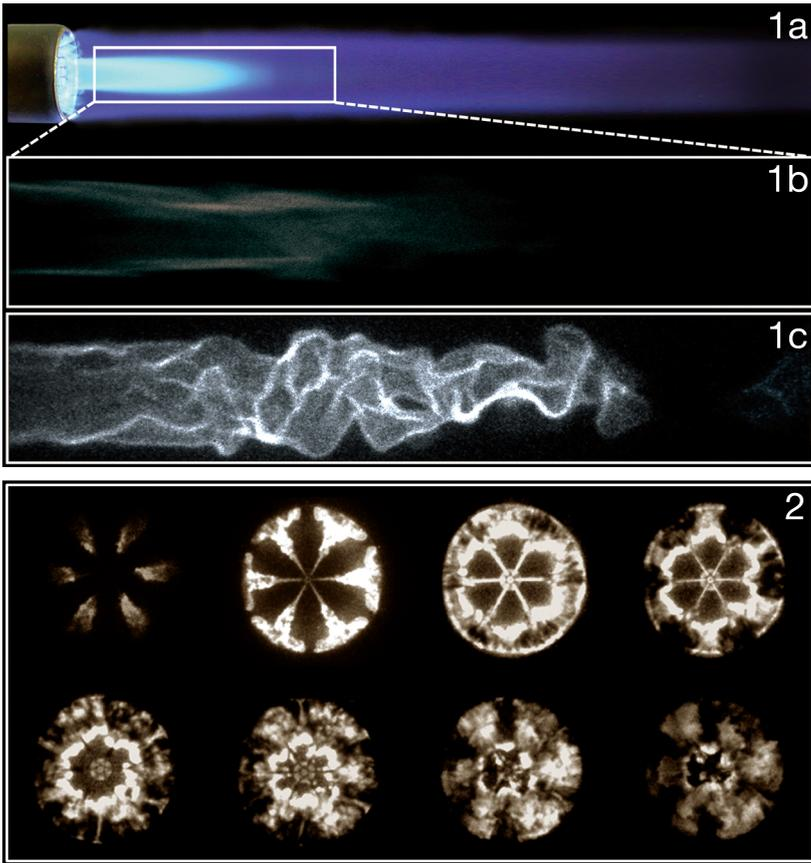
1a. Recording a blue gas flame from a Bunsen burner at high frame rates poses a challenge. The light intensity of the flame is low and to be able to see any details, especially in close-ups, very short exposure times are required.
