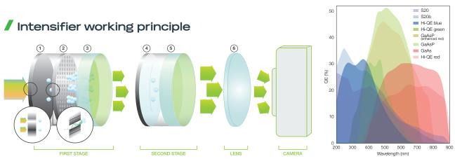
On the photocathode (1) photons get converted into electrons. These are accelerated in an electric field towards the Multi Channel Plate (MCP) (2) and hit the channel walls. Depending on the voltage across the channel, multiple electrons are generated by secondary emission. This cloud of electrons gets accelerated towards the anode screen (3), where the electrons are converted back into photons by the phosphor layer,
