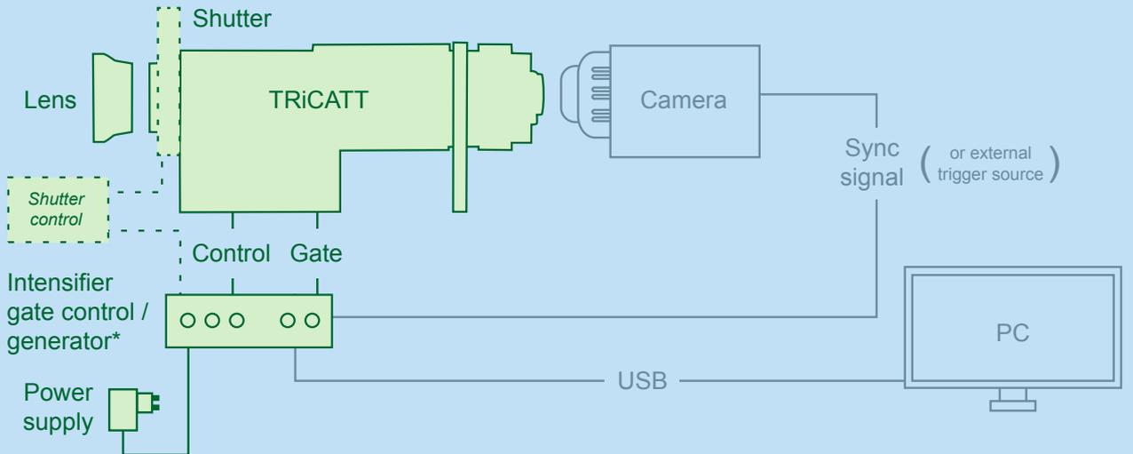
\*The intensifier gate generator can also operate as master trigger source for camera, intensifier and other devices
