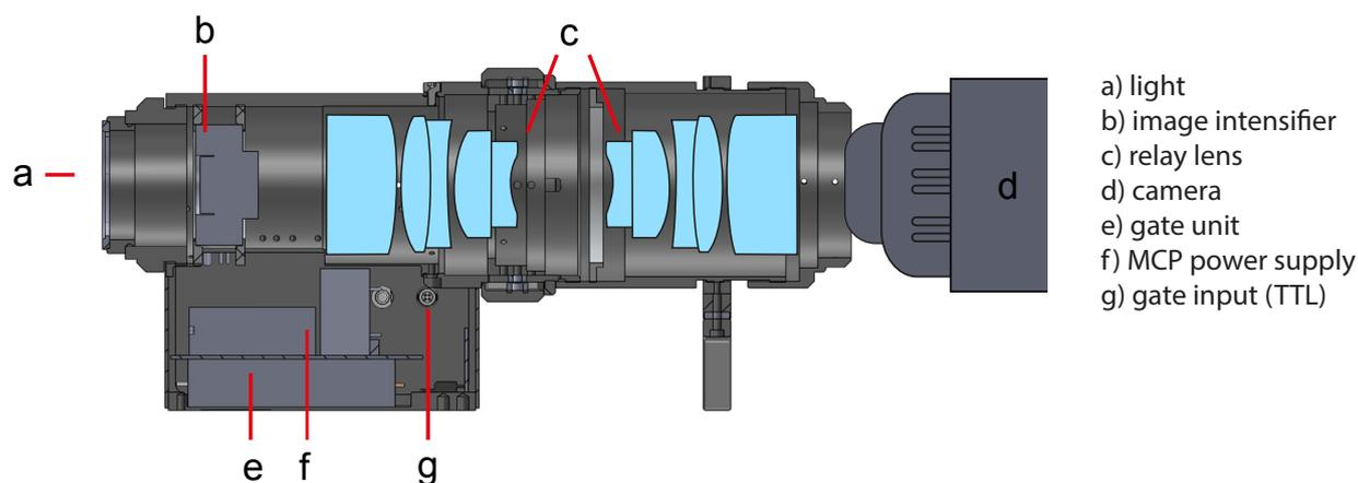
When the TRiCATT is mounted to a lens or microscope, the incoming light (a) is focused onto the entrance window of the image intensifier (b). The image intensifier converts the optical image to electrons at the photocathode, amplifies this electron image at the micro-channel plate (MCP), and re-converts the electrons into photons at the anode screen. At the output of the intensifier, a relay objective is mounted with a magnification that matches the intensifier to the high-speed camera sensor.
