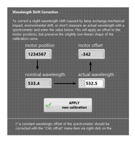
When you click on "APPLY new calibration" the calibration table will be changed accordingly.
