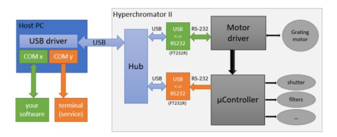
Only the COMx port is used to control the device, with the motor driver occasionally forwarding some setand-forget commands like "open shutter" to the  $\mu$ Controller. Thus, the motor driver does not receive any response from the  $\mu$ Controller. In current hardware it is not implemented to receive a "shutter open position reached" signal. Rather one must set a reasonable delay, typ. 300ms, before issuing further actions.
