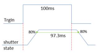
This effect will cause the dose of light emitted to show a certain deviation from linearity. For example, a 200 ms emission would have a slightly more than double dose of light. This depends also -to a small amount-on the fiber diameter connected to the instrument. Thus, for the highest precision required it would be advised to calibrate the exposure time by independent means. This may, for example, be a photodetector with fast and linear response and an oscilloscope.
