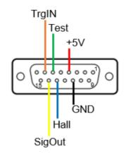
A bifurcated cable for the option port has been provided as a starting point giving access to the control lines of the HSS. The option port is also being used for switching on the XWS-30 light source as a slave device by sensing the Hyperchromator's +5 V vs GND. Should you require to modify the cable, please keep these 2 wires.
