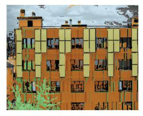
Example of hyperspectral imaging for remote sensing. The image shows the result of a classification algorithm, which distinguishes the sky (light blue), the buildings (orange), the tree (and their reflections in the windows of the building, in green) and the solar panels (in yellow).
