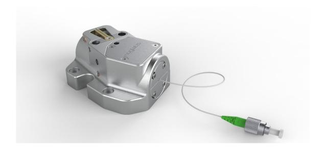
The MOGLabs CES cateye laser combines the advantages of cateye filter technology with unique butterfly-packaged single angled facet laser diodes. The CES achieves extremely low linewidth (5 kHz) and very broad tuning range, with integral Faraday isolator and fibre-coupled output.
