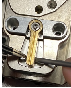
Figure 4.1: Removing the intracavity filter assembly.
