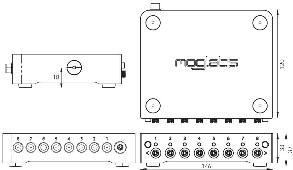
Figure F.2: FSW fibre switch dimensions.
