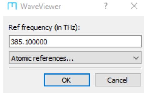
**Figure 6.8:** Dialogue to specify the exact frequency of the reference laser (in MHz). Select from the atomic references, or enter a frequency in MHz. Enter zero to use the average of the first 25 measurements as the reference.
