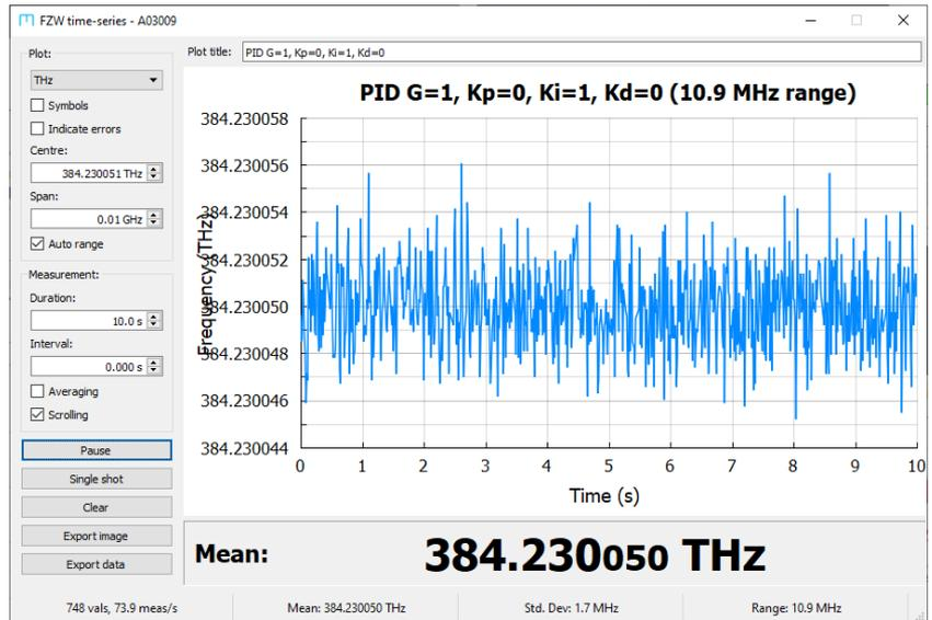
**Figure 5.6:** Fluctuations in the measured laser frequency when locked. These fluctuations are at the limit of the measurement of the position of the longest etalon fringes: a few MHz in a fringe spacing of 7500 MHz.
