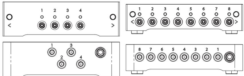
**Figure 6.2:** FSW4 (left) and FSW8 (right) optical switches. The front-panels (top) have fibre inputs and LED indicators, while the back-panels (bottom) have SMA outputs for monitoring and PID control. The front-panel buttons cycle between the input fibres.
