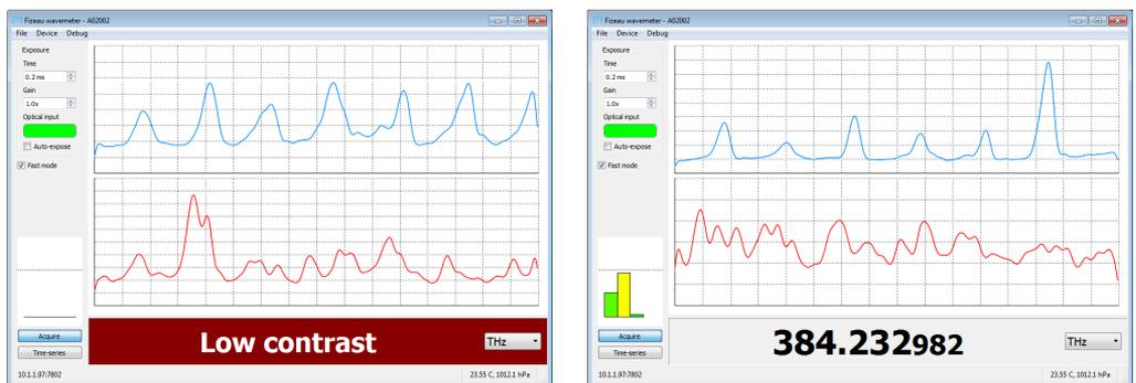
Figure 4.4: Examples of fringes measured with a 200  $\mu\text{m}$ -core fibre. The mode shape makes reliable readout almost impossible (left) although in some situations a low-accuracy measurement can still be achieved (right).
