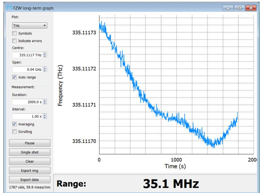
**Figure 3.5:** The time-series window shows how the wavelength measurement is changing over time, for measuring drift. The graph displays *Duration* seconds of data, with a datapoint collected every *Interval* seconds. When *Averaging* is enabled, the wavelength measurements during each interval are averaged to enhance the measurement precision.
