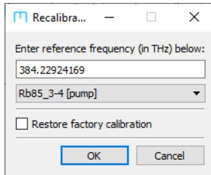
**Figure 4.7:** The recalibration window of the host software allows correction of the device calibration using a known reference. A standard reference can be selected from the dropdown box, or a custom reference frequency can be entered.
