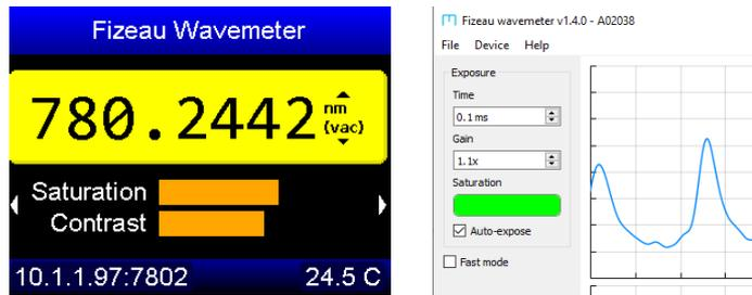
**Figure 1:** Both the built-in wavemeter display (left) and host software (right) provide saturation indicators that measure the optical power reaching the detector.
