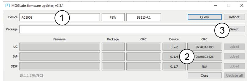
**Figure B.1:** The firmware update application connected to a FZW unit, showing the device serial number (1) and current firmware versions (2). Click the *Select* button (3) to open a firmware package for upload.
