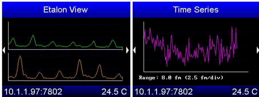
**Figure 3.2:** Diagnostic modes of the FZW device UI: etalon display (left) permits verification of fringe quality, and time-series display (right) shows variation in the measured wavelength over time.
