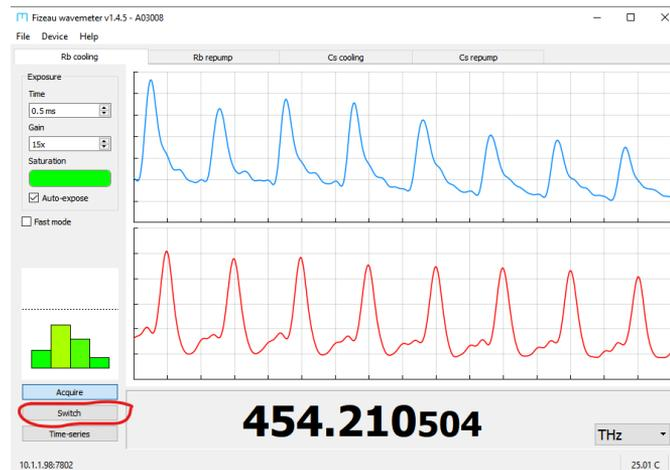
**Figure 6.4:** With FSW connected, the PID button in `mogfzw` is replaced with a `Switch` button that opens a new dialogue for monitoring and controlling the switch channels.
