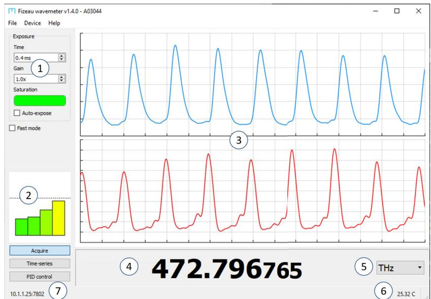
**Figure 3.4:** Demonstration of the host software interface, showing exposure controls (1), convergence monitor (2), interference fringes (3), measured wavelength (4), display units selector (5), etalon temperature (6) and communication address (7). The font size of the measured wavelength can be enlarged by dragging the splitter bar vertically.
