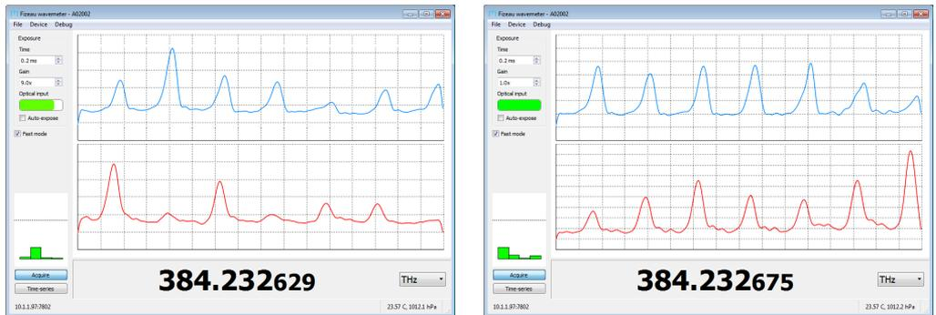
Figure 4.3: Example fringes measured with a 62.5  $\mu\text{m}$ -core fibre demonstrating envelope structure that causes measurement bias (left). Adjusting the input coupler alignment can give more uniform fringe heights (right) and more reliable measurement.
