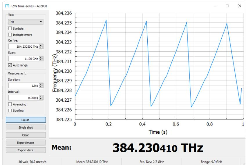
**Figure 3.6:** The FZW can be used to measure the mode-hop free scan-range of a laser. Setting the *Interval* to zero ensures measurements are recorded as rapidly as possible. The measurement rate, measurement mean, standard deviation and peak-to-peak range are shown in the status bar at the bottom.
