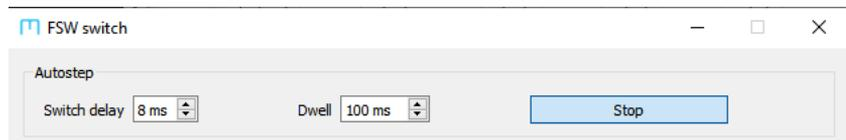
Figure 6.6: Control of auto-stepping via the `F5W switch` control window.
