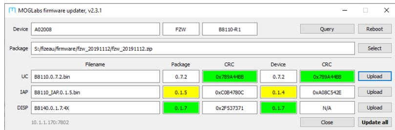
**Figure B.2:** The firmware update application with a loaded package. The versions running on the device are compared against the selected package, in this instance showing that an update is available for the IAP (yellow) and the other components are up-to-date (green).
