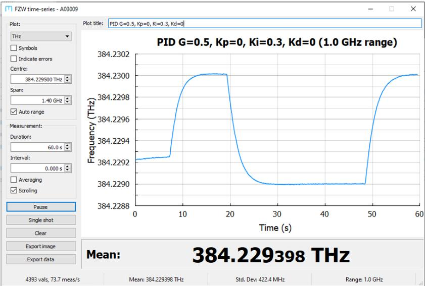
Figure 5.4: Time series measurement of the wavelength when PID is enabled at about 8 s. The setpoint is changed at around 20 s and again at 48 s.
