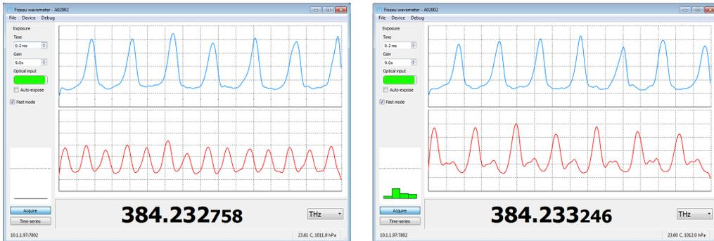
**Figure 4.2:** A multimoding laser might only be evident in one of the interference patterns. In some circumstances this will be clear from an obvious change in fringe spacing (left), whereas at other times the secondary peaks might be smaller amplitude (right).
