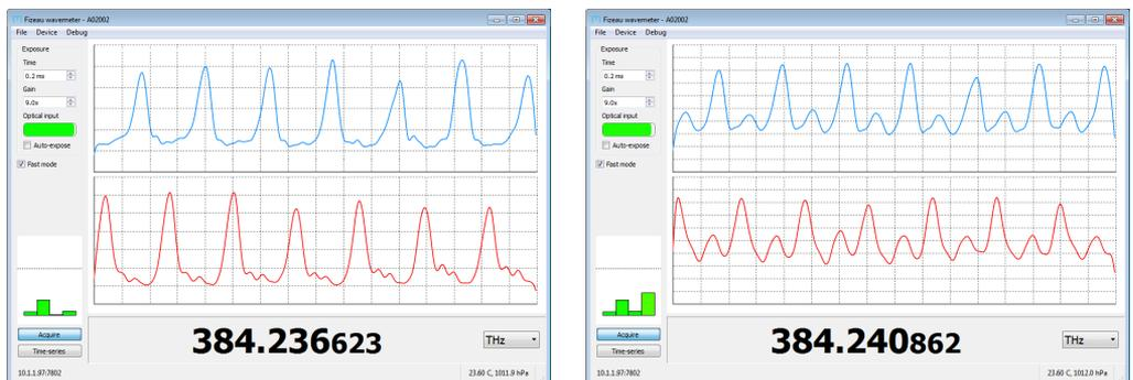
**Figure 4.1:** Examples of fringes measured with a single-mode laser (left) and multimode laser (right). The presence of secondary peaks and reduction in contrast indicate the laser is not single-mode.
