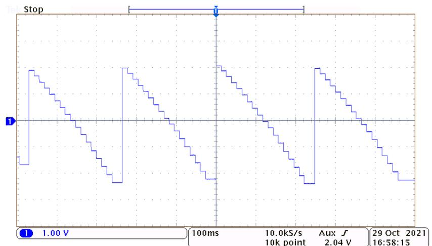
**Figure 5.3:** Wavelength measurement of a scanning laser. The gain was set to 0.5V/GHz and the ramp amplitude shows that the laser was scanning 9GHz. Note that the discrete steps are due to the measurement time, about 15ms per sample, not digitisation of the DAC.
