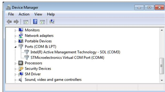
**Figure E.2:** Screenshot of Device Manager, showing that the FZW can be communicated with using COM4. The port number might change when plugging into a different USB port, or after applying a firmware update.
