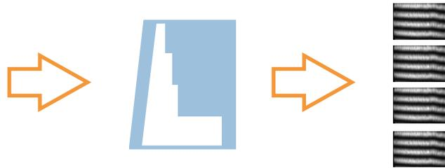
**Figure 1.1:** Collimated monochromatic laser light and Fizeau etalons create interference patterns on an imaging detector. The wavelength is calculated by combining measurements of the fringes from four different etalons.
