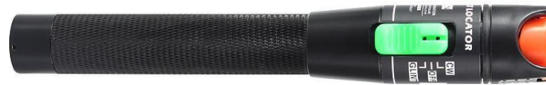
Figure 7.2: Visual fault locator (VFL). Injects visible laser light into a fibre, allowing initial alignment and mode matching.
